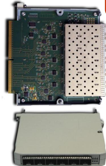
Figure 2: Custom developed FlexRIO Adapter Module with 6 fiber connectors
