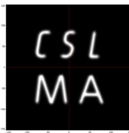
Fig. 4: Beam scan, delivered with a C-DDS prototype at MedAustron
